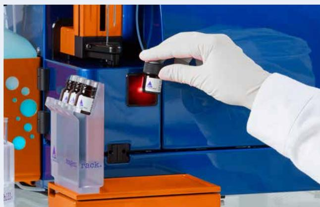
Figure 3: Reagent scanning for easy autolabeling.
