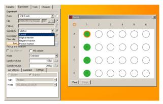
**Figure 8:** In order to change the default sample IDs activate the sample well and choose a sample ID from the pull-down menu.
