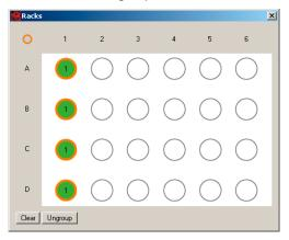
**Figure 7:** Rack positions A1 – D1 have been assigned to group 1 by using the group function.
