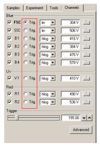
**Figure 2:** Select the channel for the trigger to be used by checking the trigger button.
